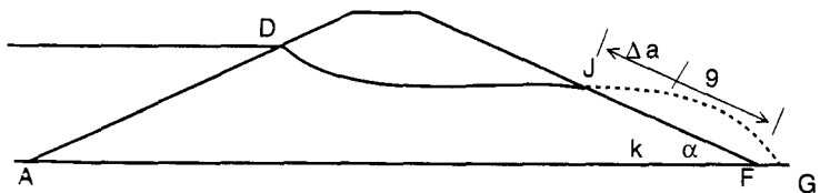
Gb. 6.58. Bendungan tanah tanpa filter drainase.
